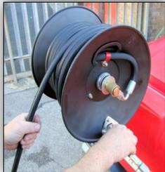
Release pin on hose reel and wind hose in and replace pin.
