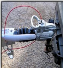
Release handle to lock into place around ball hitch.
