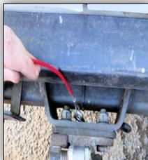
Unlock safety brake cable & thread around tow bar.
