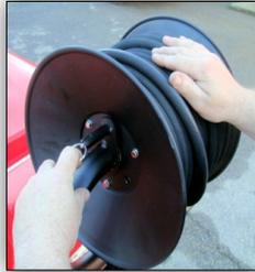
Pull pin on hose reel to release hose.
