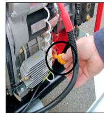
Check the engine oil. Replenish as required.
