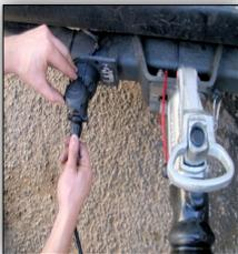
Attach the lighting board plug to socket on tow bar.
