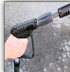
Release any pressure in the hose by squeezing the trigger.
