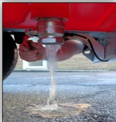
Turn the handle to the downward position and the water will release.
