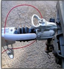
Place the tow hitch over the ball hitch on the tow bar
