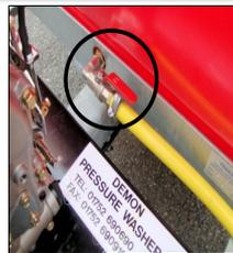
Check ball valve is in the 'on' position.
