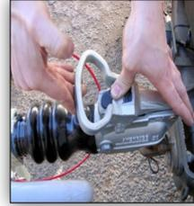
Hold up bowser handle, push button and lift hitch to release lock.
