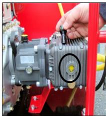
Check the oil in the pump – using dipstick or sight level
