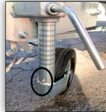
Turn jockey wheel clamp anti-clockwise until pin in place with U
