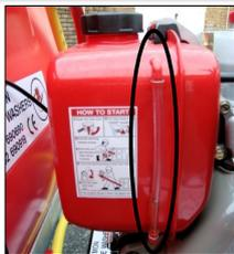
Check diesel using sight level and fill as required.
