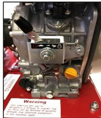
When finished working pull lever back to tortoise 'stop' position.
