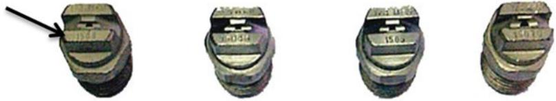
Pressure starts and ends at the nozzle. The volume of water pushed down the hose and forced through the small hole determines the pressure on the gauge. Try taking the nozzle out and then pulling the trigger. You get virtually no pressure registering on the gauge.
