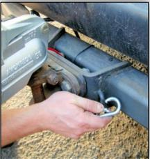
Attach to tow bar ring if possible or back around safety brake cable.
