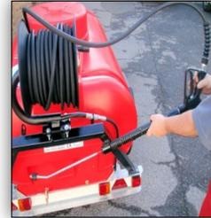
Remove lance from holder and pull hose off to desired length
