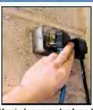
Unwind power lead and plug into mains. NB not an extension lead
