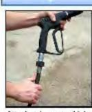
Attach trigger to high pressure hose.
