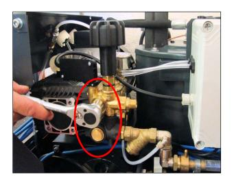
**2.** Undo the bolts which hold the unloader valve on, using a 17mm socket for the top banjo bolt and a 19mm socket for the lower banjo bolt.
