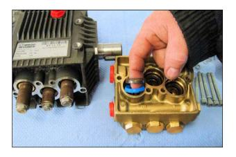
**6.** Remove the brown seal and blue back up ring from the head.
