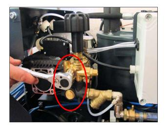
**15.** Rebuild unloader valve by placing on head ensuring the o-rings are in place in unloader valve. Do up bolts tightly on top and bottom.
