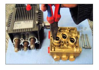
**5.** Remove the seal carriers from the pump head or from the pistons if they have got stuck on them.
