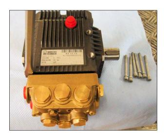
**4.** Once allen bolts are all removed separate the pump head from the pump ensuring not to damage the pump or head. Then gentle prise apart .
