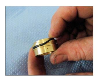
**8.** Take the piston guide and the black outer O'ring and place on the outside of the piston guide in the groove. Repeat for all 3 piston guides.
