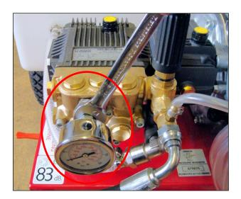
. Reconnect pressure gauge and tighten using a 17mm spanner.
