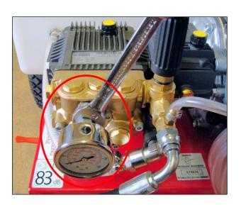
**2.** Take off pressure gauge using a 17mm spanner to gain access to allen bolts.
