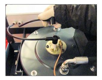
**18.** Replace HT leads back onto electrodes.
