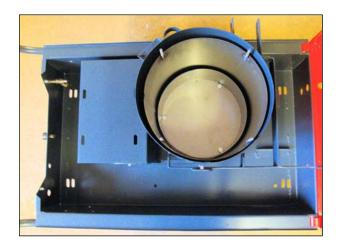
**12**. Take your assembled drum and flame pan and place into the outer boiler housing. Securing with the M10 washer and nyloc underneath the chassis.
