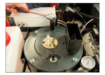
**7.** Unscrew 3/8" lock nuts using 22mm deep socket.
