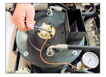
**17.** Reconnect copper fuel pipe with 8mm spanner ensuring it is tight.
