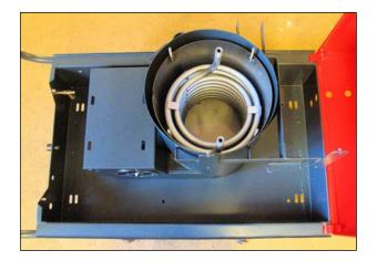
**13.** Place the coil into the stainless steel pan.
