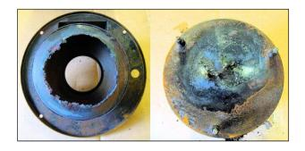
This picture shows the kind of damage which is caused to the stainless steel pan and cone through using dirty fuel and not servicing regularly.
