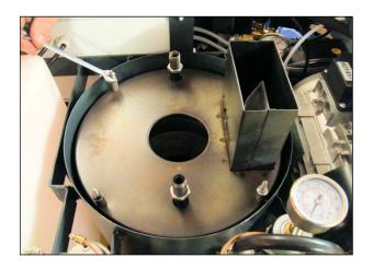
**9.** Unscrew the M6 nuts and spacers using a 10mm spanner.
