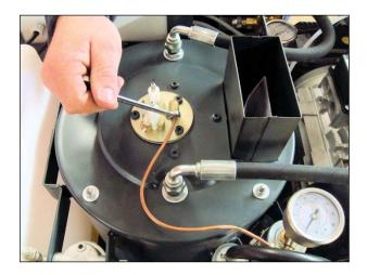
**4.** Disconnect the copper fuel pipe using an 8mm spanner and move to one side.
