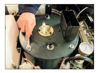
**6.** Unscrew M6 Nyloc nuts using a 10mm spanner.
