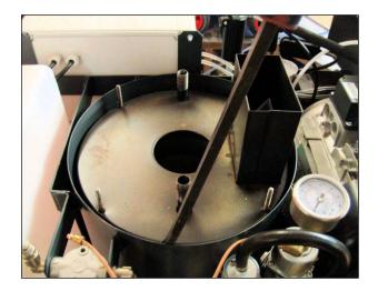
**11.** Use a pry-bar or screwdriver gentle remove the inner lid and cone to expose the coil, inner lid and stainless steel pan and replace if required.
