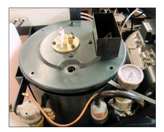
**15.** Place the lid back on and secure 3/8" and nyloc nuts which were taken off.
