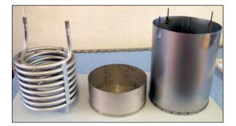
**1.** Assemble the inner drum and stainless steel pan using 3 x M10 x 70mm bolts, place stainless steel pan into the inner drum assembling spacers on the outer drum and tighten nuts from underneath.
