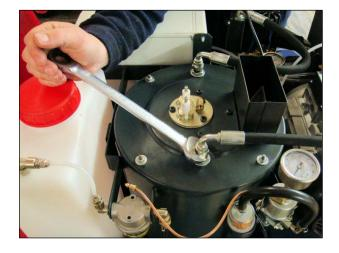
**5.** Disconnect both High Pressure Hoses from the boiler using a 22mm spanner.
