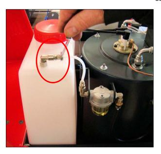
**1.** First disconnect the fuel tank from the fuel line using a 10mm spanner.
