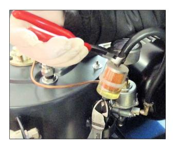
**5.** Moving to the inline filter, break top and bottom one-eared clamps and remove inline filter replacing with a new one. Ensure that the arrow is pointing upwards towards pump when replacing filter. Replace with one-ear clamps ensuring a good seal.
