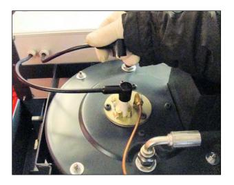
**18.** Replace HT leads back onto electrodes.
