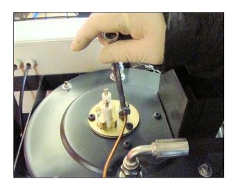
**17.** Reconnect copper pipe with 8mm spanner ensuring it is tight.
