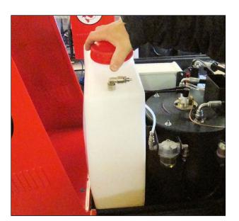
**2.** Remove the tank and dispose of the dirty fuel in a safe method. Clean the fuel tank using hot soapy water to ensure all residue is removed.
