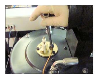
**11.** Disconnect copper fuel pipe with an 8mm spanner and move to one side.
