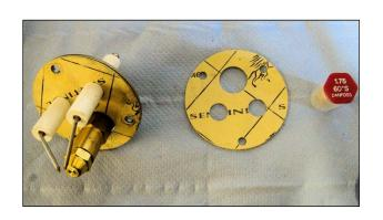
**13.** Remove nozzle with a 16mm spanner and remove gasket and replace with new ones.
