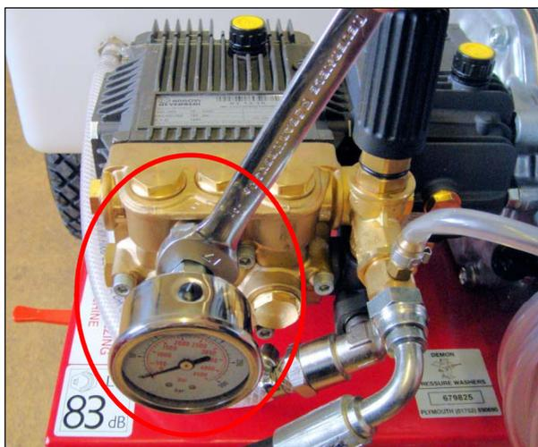
**15.** Reconnect pressure gauge and tighten using a 17mm spanner.
