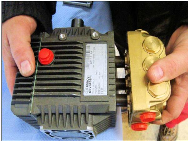
**13.** Push the head back onto the pump. If it appears to be tight, then gently tap with a hammer to ease onto pistons.
