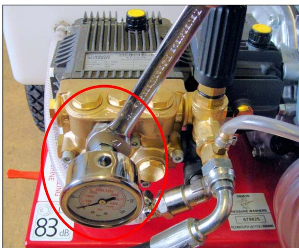
**2.** Take off pressure gauge using a 17mm spanner to gain access to allen bolts.
