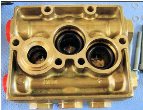
**12.** Take seal carrier with o-rings in place and apply a thin layer of silicon grease around the outer o-ring. Push into the head ensuring not to nick the o-ring. Repeat for all 3.
