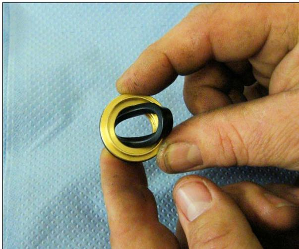
**9.** Take the inner plastic black seal and place inside the piston guide. Repeat for all 3 piston guides.
