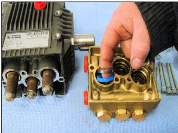
6. Remove the brown seal and blue back up ring from the head.
