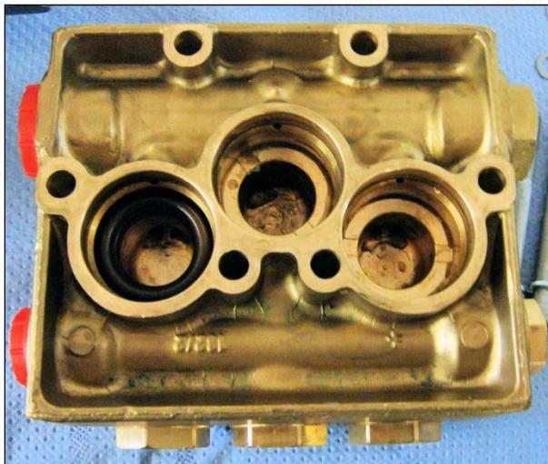
**11.** Take the brown seal and place on top of the blue back up ring, pushing it into place. Repeat for all 3.
