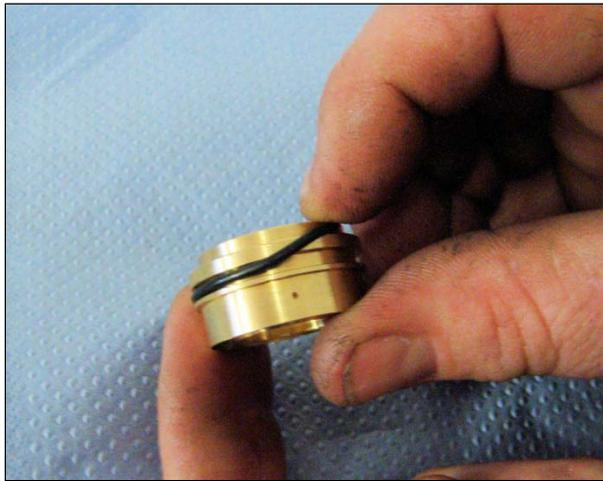
**8.** Take the piston guide and the black outer O'ring and place on the outside of the piston guide in the groove. Repeat for all 3 piston guides.
