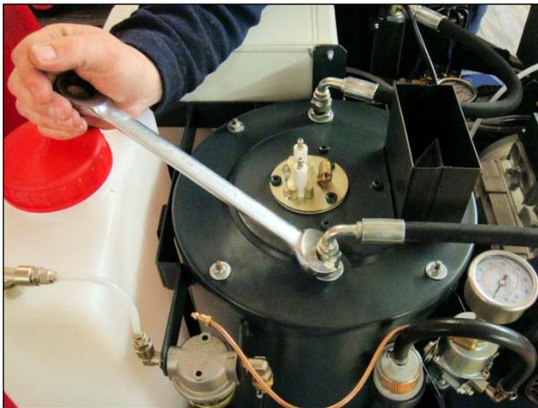
**16.** Reconnect high pressure hoses to the top of the burner using a 22mm spanner.
