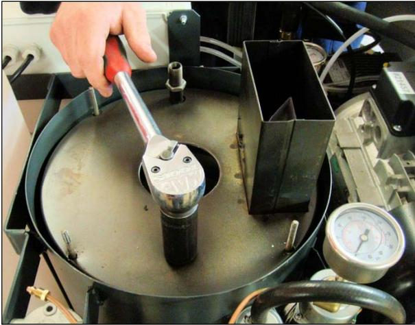
**10.** Unscrew the inner 3/8" lock nuts using a 22mm deep socket.
