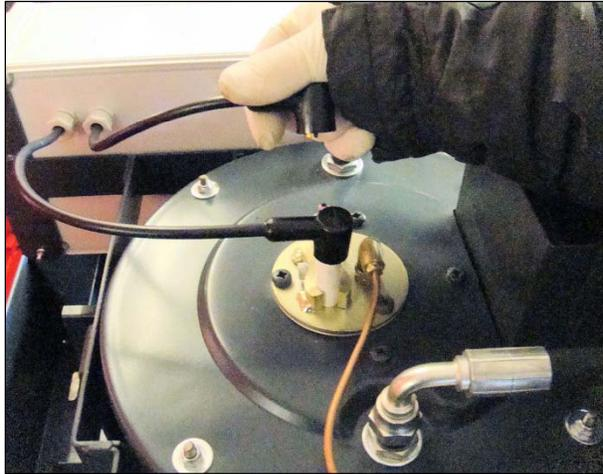
**18.** Replace HT leads back onto electrodes.
