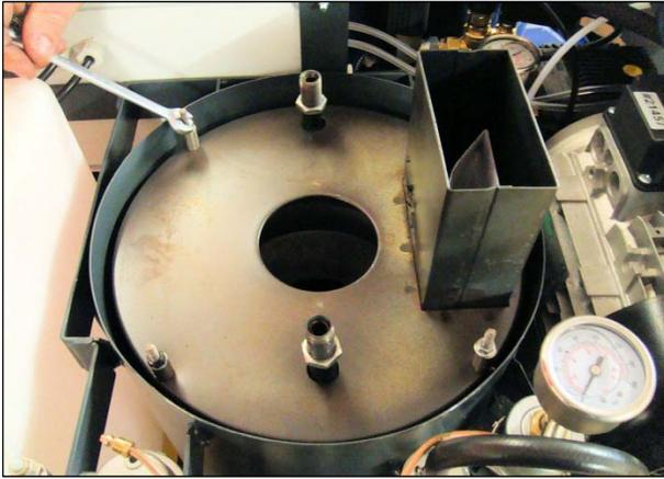
**9.** Unscrew the M6 nuts and spacers using a 10mm spanner.
