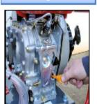
Check engine oil and replenish as required.
