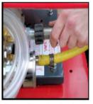
Place filter in bucket or water source & connect hose to machine & tighten
