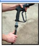
Attach trigger to high pressure hose.
