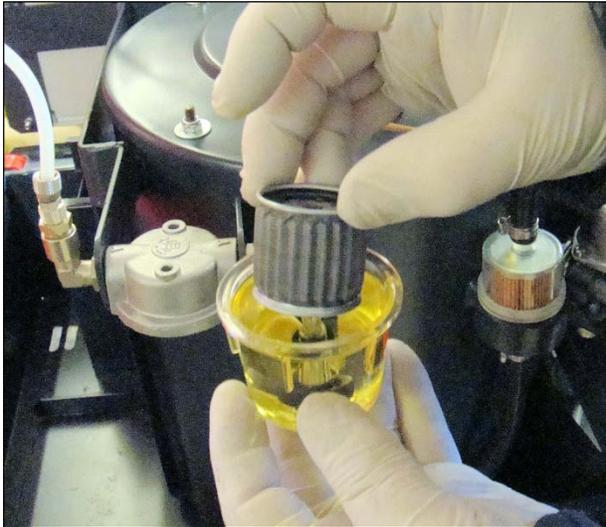
**4.** Clean the filter and bowl using hot water and screw back into position ensuring that the filter and bowl are dried or blown away with a compressed air supply.
