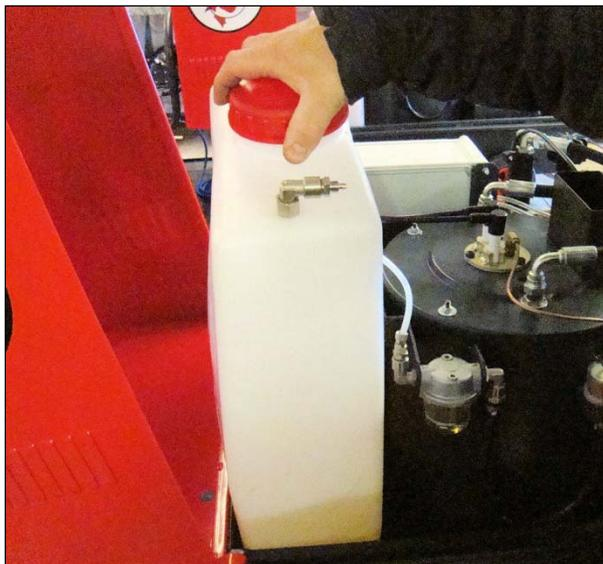
**2.** Remove the tank and dispose of the dirty fuel in a safe method. Clean the fuel tank using hot soapy water to ensure all residue is removed. Make sure all traces of water are removed before replacing.
