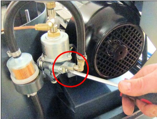
**19.** You will then need to run the machine up to bleed the pump and obtain pressure on the gauge between 100-110 psi to ensure the correct burn.
