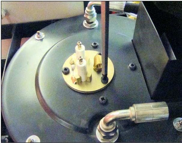
**12.** Unscrew the 3 x M6 screws holding burner head in place and remove.
