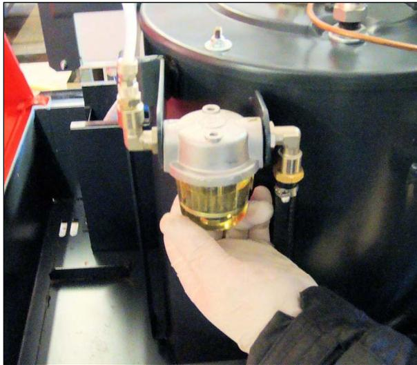
**3.** Moving to the fuel filter bowl, unscrew the filter bowl and remove aluminium filter.
