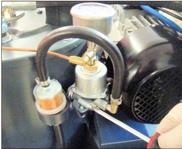
**6.** Moving on to the fuel pump, unscrew the 2 screws which hold the fuel pump plate-where fuel pump sits behind.
