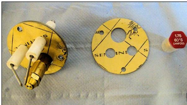
**13.** Remove nozzle with a 16mm spanner and remove gasket and replace with new ones.
