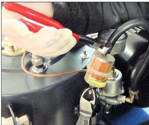
**5.** Moving to the inline filter, break top and bottom one-ear clamps and remove inline filter replacing with a new one. Ensure that the arrow is pointing upwards towards pump when replacing filter. Replace with one-ear clamps ensuring a good seal.
