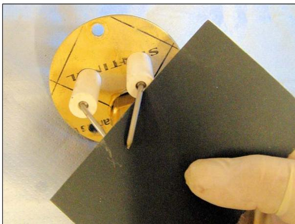
**14.** Clean electrodes with a small piece of sandpaper. If electrodes are damaged or show sign of movement then replace with new ones.
