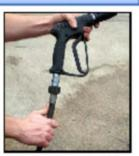
Attach trigger to high pressure hose.
