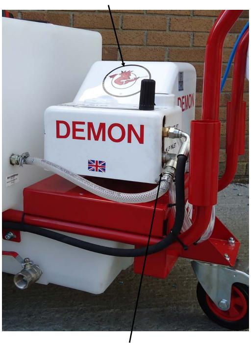
Inlet Fittings DEM20441 3/8 X 1/2" Hose tail MTM0012FF03 Brass elbow 1/2FF
