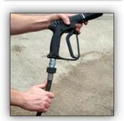
Attach trigger to high pressure hose.
